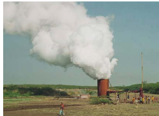
Figure 2: Production test of well TD5 (at well head: T > 250\text{ °C} , p > 18\text{ bar} ). The well is located inside the MT survey area.
