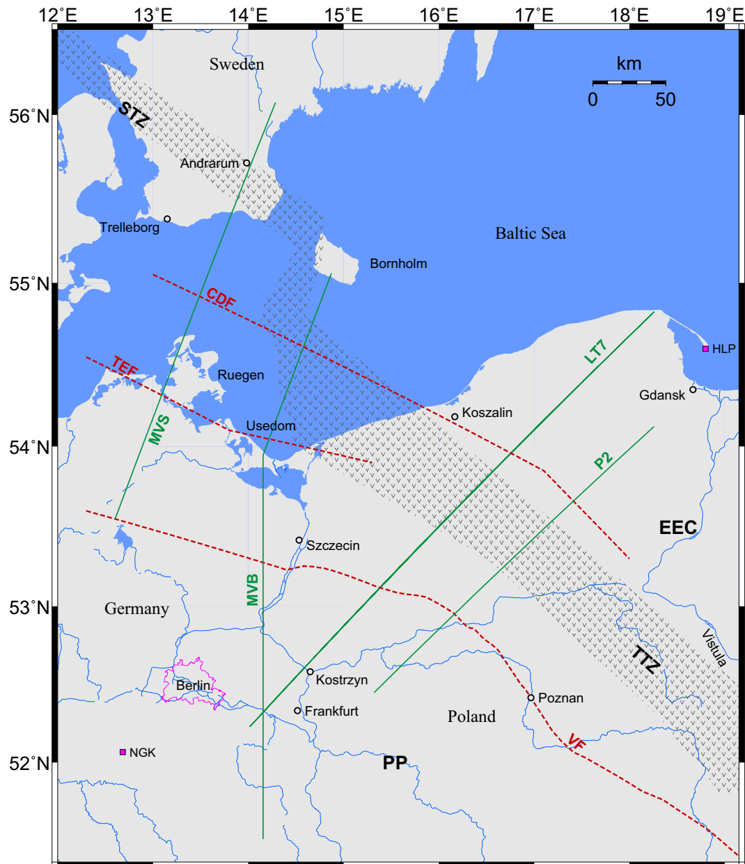
Figure 1: Overview of measurement area with profiles P-2, LT7, MVB, and MVS. Important tectonic elements are the Trans-European Suture Zone (TESZ) consisting of the Sorgenfrei-Tornquist Zone (STZ) and the Teisseyre-Tornquist Zone (TTZ), the Caledonian Deformation Front (CDF), the Trans-European Fault (TEF), the Variscan Front (VF), the Precambrian Platform or East European Craton (EEC), and the Paleozoic Platform (PP).
